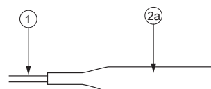
Style 34 1: 75 cm capillary 2: 1/4" tube for braze connection
