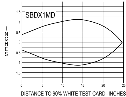
Figure 10. Beam Pattern - SBDX1MD
